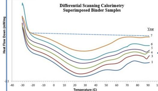
**DSC** scans of wax/oil binder showing a decrease in melting enthalpy over time. The successive enthalpy decrease suggests a decrease in crystallinity over time which correlates with the scissioning/fracturing of larger molecules observed in the GC-FID results.
