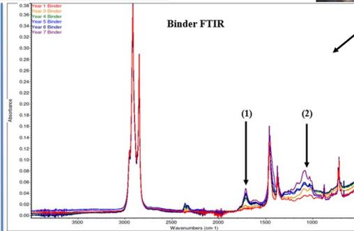
**Fourier Transform Infrared Spectroscopy (FTIR)** results clearly reveal increasing oxidation over time in the 1700  $\text{cm}^{-1}$  carbonyl peak wavelength region (2). This oxidation activity is common to aged oils and can be seen in this study to be occurring predominantly within the oil in the wax binder.
