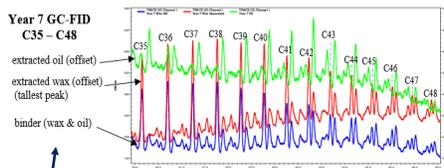
**Gas Chromatography:** Wax binder GC-FID comparison of Year 1 and Year 7 gas chromatography spectrums (top two). Year 1 and 7 extracted wax and extracted oil C35 to C38 spectrums are expanded and superimposed to show distinct trailing peaks not present in Year 1 binder spectrum. In the offset oil scan, the only peaks present are trailing peaks, indicative of oxidized, potentially polar molecules that increase substantially over time
